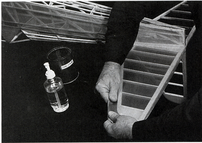
Pull the silk gently spanwise and chordwise along the remaining edges to eliminate wrinkles, doping it down as you go.
