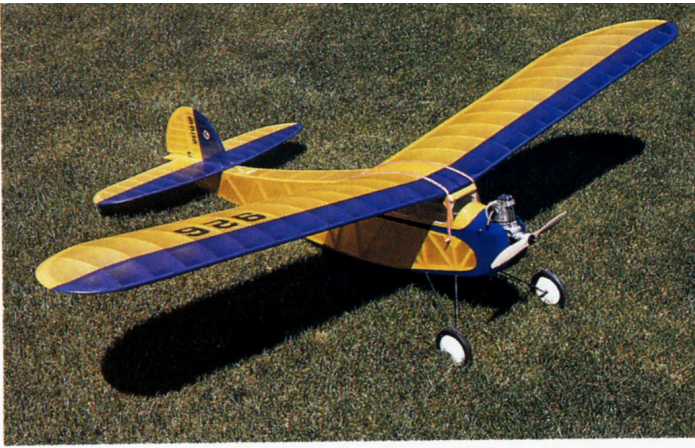
Author Munn's 84-inch-span Powerhouse is covered in yellow and blue silk, and uses an O.S. .61 four-stroke engine.
