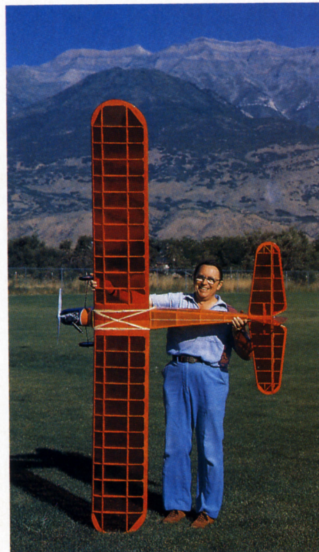
Robert Munn's 9-foot-span red Dallaire Sportster uses an Enya .90 four-stroke. Finish is Sig clear butyrate.
